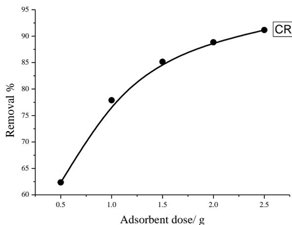
Fig. 3. Effect of adsorbent dose on percentage removal of CR [Initial conc.=20 mg/L, Time of adsorption=24 hrs., Temp=302k,pH=6.28, volume of adsorbate=50 ml].
