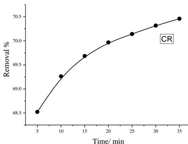
Fig. 2 Effect of contact time on percentage removal of CR, [Initial conc.= 20 mg/L, Adsorbent dose=1.0 g, temp = 298.3 k, pH = 5.87].
