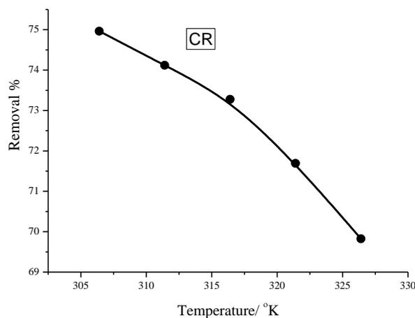
Fig. 6 Effect of temperature on percentage removal of CR [Initial conc.=20 mg/L, Adsorbent dose=1.0 g,volume=50 ml,pH=6.12, time of adsorption=24 hrs.].
