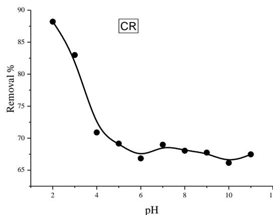
Fig. 5. Effect of pH.on percentage removal of CR [Adsorbent dose=0.5 gm, Initial Conc.=20 mg/L., Temp=301.5k,volume of adsorbate=25 ml.]
