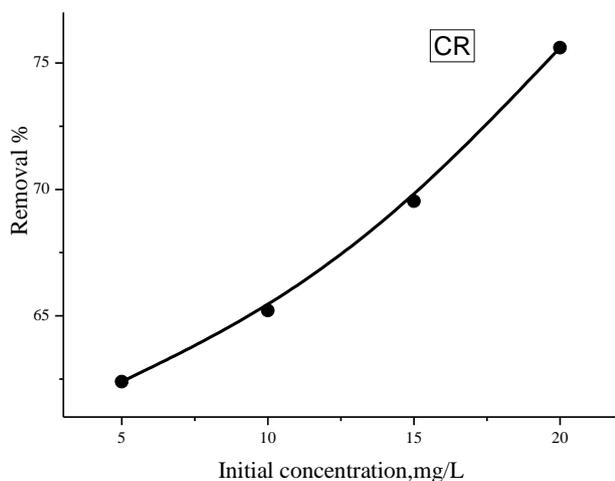
Fig. 4 Effect of initial conc.on percentage removal of CR [Adsorbent dose=1.0gm., Time of adsorption=24 hrs. Temp=298.3k,pH=6.14, volume of adsorbate=50 ml].
