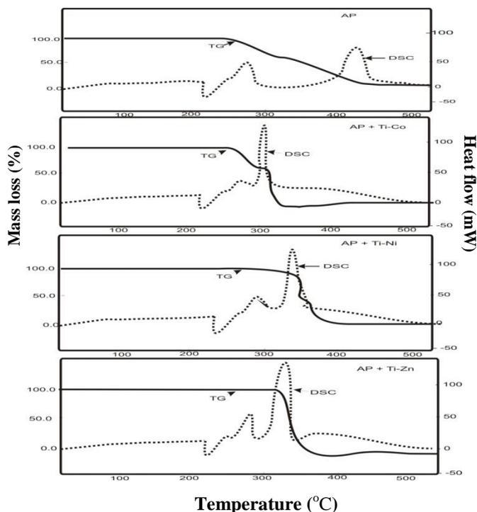
Ti-alloys nano-alloys are shows potential catalytic effect for thermal decomposition of ammonium perchlorate at much lower temperature.
