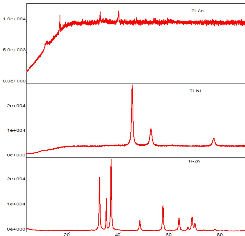
Fig. 1 XRD Pattern of Ti-alloys
