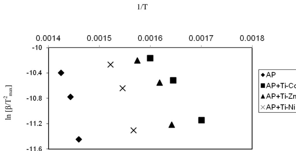
Fig. 4 Plot of  $\ln(\beta/T^2_{max})$  versus  $1/T$  for AP and AP with BMNs
