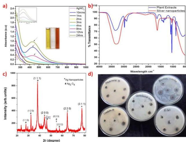
Figure 2 a - UV/Vis Spectrophotometer analysis of synthesized silver nanoparticles; b - FT-IR characterization of synthesized nanoparticles and plant source (extract); the XRD pattern of Ag nanoparticles prepared by plant extract as presented in Fig - c; d - Antimicrobial assay of silver nanoparticles using well diffusion assay method.
