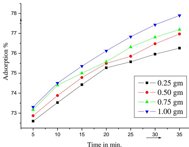
Nickel (II) metal ion adsorption at Red gram seed husk depends on initial concentration of metal ion, adsorption dose, temperature etc.
