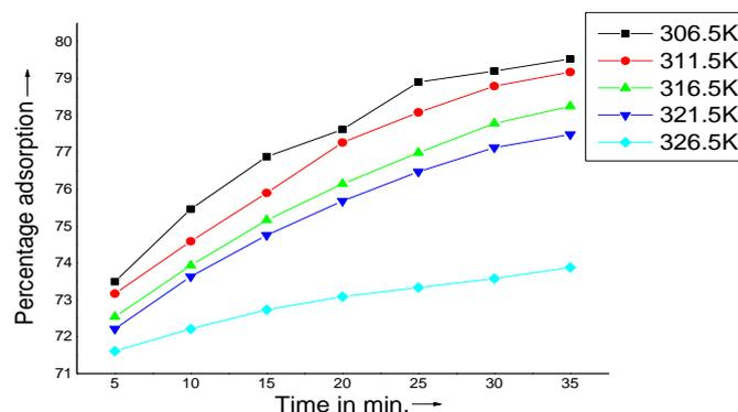
Fig. 4: Effect of temperature on percentage adsorption of Ni(II) [Initial conc. = 20mg/L, Adsorbent dose = 0.5gm, pH = 5.9]
