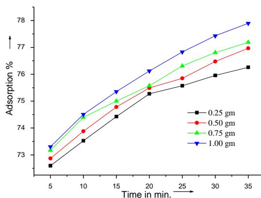
Fig. 2 effect of adsorbent dose on percentage adsorption of Ni (II), [Initial conc.= 20 mg/L,Temp=304.5k,pH=5.9]
