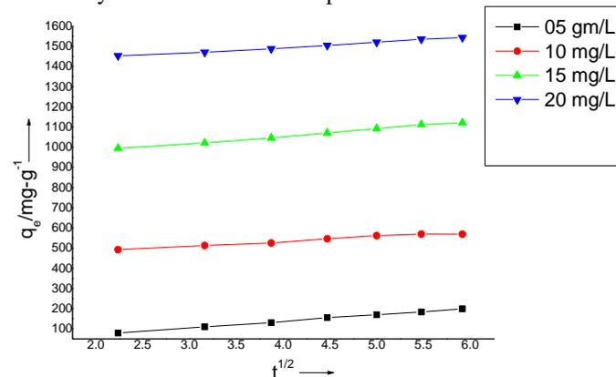
Fig 4. : Plot of  $q_t$  against  $t^{1/2}$  in internal diffusion model with Initial concentration of Ni (II) metal ion
