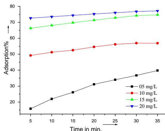
Fig. 1 effect of contact time on percentage adsorption of Ni(II) [Adsorbent dose = 0.5 gm, Temp = 304.5k, pH = 5.9]
