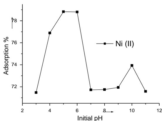
Fig. 3: Effect of initial pH on percentage adsorption of Ni (II) [Initial conc. = 2.0mg/L, Volume – 2.5ml, Temp. = 304.5K]
