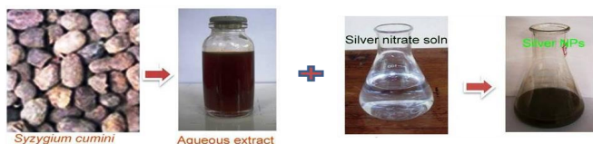
Fig 1: preparation of AgNPs using Syzygium cumini seed endosperm aqueous extract.
