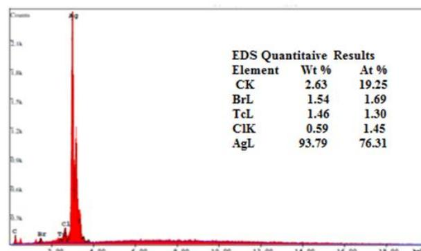
Fig. 6. Energy dispersive X-ray spectrum (EDS) of silver nanoparticles.
