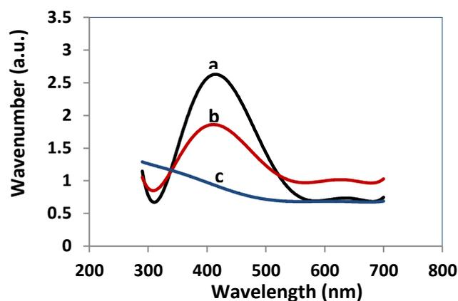
**Fig. 1.** UV-vis absorption spectra of silver nanoparticles as a function of time for reaction of 1mM aqueous solution: a = 1 min, b = 0.5 min, and c = *Ailanthus altissima* leaves extract.
