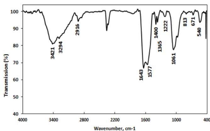
Fig. 4. FT-IR spectrum of synthesized AgNPs.
