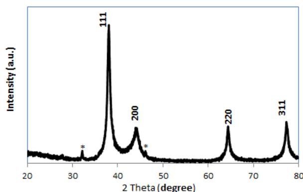
**Fig. 2.** XRD spectrum of biosynthesized silver nanoparticles.
